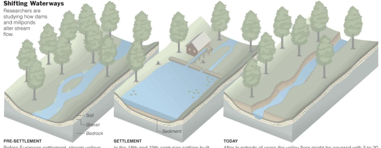
Before European settlement, stream valleys in the Middle Atlantic states were typically marshy, with shallow channels of water flowing in sheets over gravel stream beds. Source: LandStudies In the 18th and 19th centuries settlers built dams by the thousands. Trapped sediment runoff from logging and farming slowly filled in the millponds. If a dam failed another dam might be built on top of it, or just downsteam.
