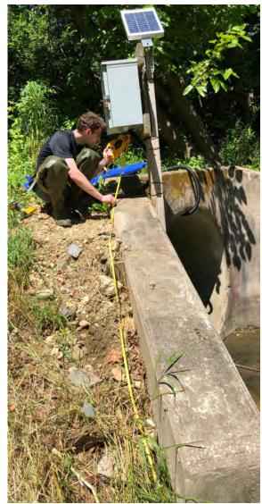
Sensors provide high-frequency nitrate & discharge data for calculating loads.
