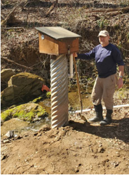
Figure 5. Photo showing stormwater monitoring station at UTLP; automatic sampler and Aquatroll 500 not visible.
