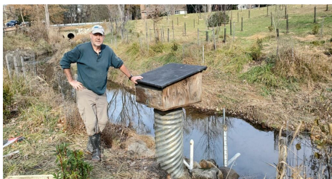
Figure 4. Photo showing stormwater monitoring station at PLBR; automatic sampler and Aquatroll 500 not visible.
