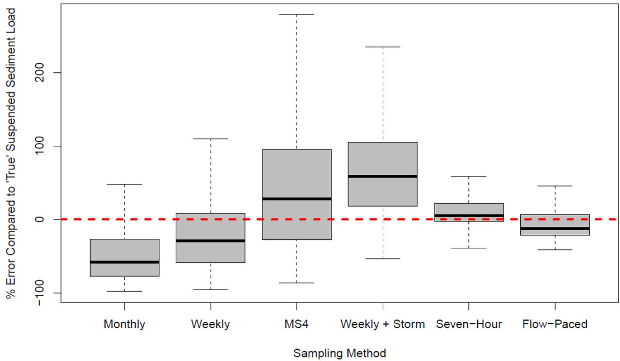
Figure 2. Relative error in SSC estimates based on various sampling frequencies compared with the load calculated from high-frequency data
