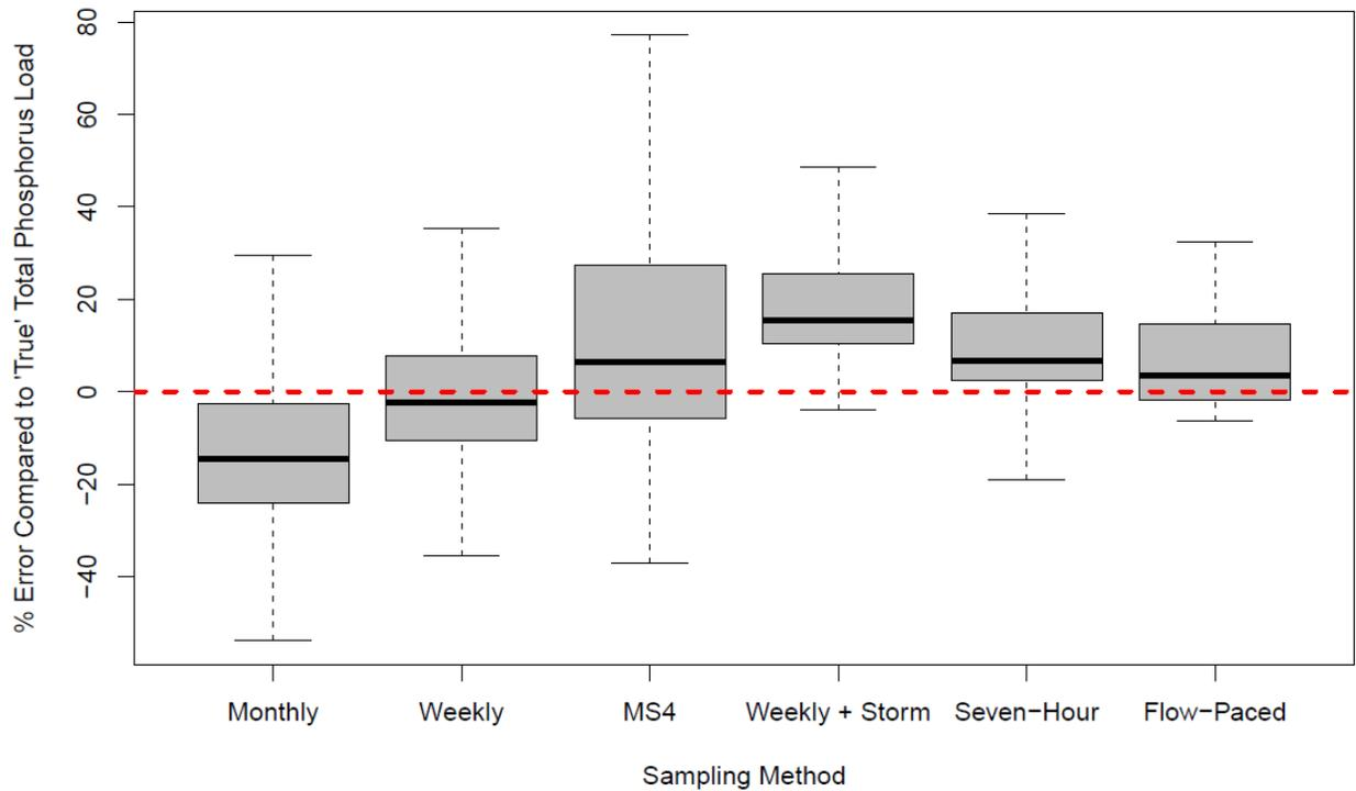
Figure 3. Relative error in TP load estimates based on various sampling frequencies compared with the load calculated from high-frequency data
