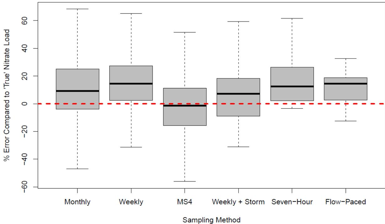
Figure 4. Relative error in nitrate load estimates based on various sampling frequencies compared with the load calculated from high-frequency data
