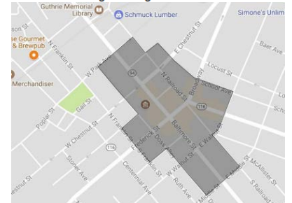
Green Alley Network - Bank Lane Pedestrian Green Alley Contributing Drainage Area: 2.54 Acres
